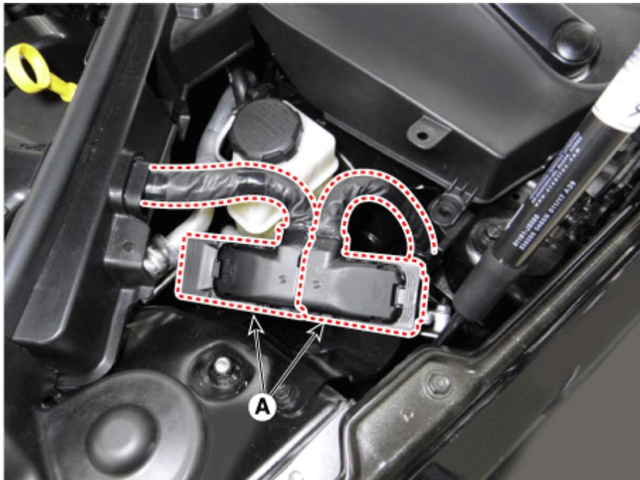
4. Remove the ECM bracket assembly after loosening the mounting bolt (A) and nuts (B).
